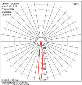
Manufacturer: FC LIGHTING Luminaire catalog: FCC610A Luminaire: FCC610A-SF-UNV-AM-4L-BKE-SP-TD-CV
