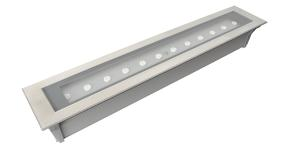
FCD7000 Linear Inground Uplight is ETL listed for wet locations. Housing is marine grade, corrosion resistant, heavy walled, high pressure aluminum construction with 316 Stainless Steel Trim (aluminum well housing included). In addition, the lens is impact resistant, clear, tempered glass. Reflector is precision formed semi-specular aluminum for maximum reflectance with LED.
