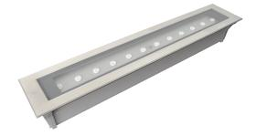
FCD7002 Linear Inground Uplight is ETL listed for wet locations. Housing is marine grade, corrosion resistant, heavy walled, high pressure aluminum construction with 316 machined brushed stainless steel trim (aluminum well housing included). Lens is impact resistant, clear, tempered glass. Reflector is precision formed semi-specular aluminum for maximum reflectance with LED.
