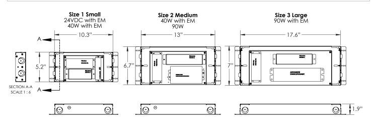
BBUX - BATTERY BACK-UP & LED DRIVER REMOTE (OUTDOOR), IP67, IK10, NEMA 4X, -20°C to +55°C, 30' MAX Distance with 12AWG (w/UNV Option Only)
