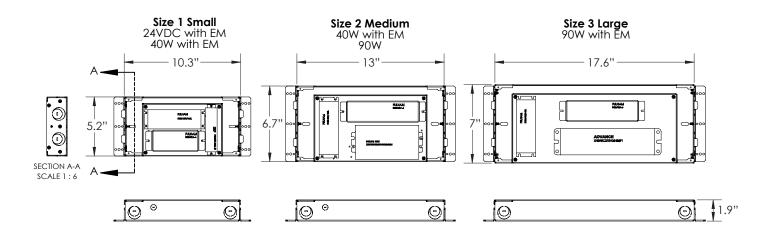
**BBUX -** BATTERY BACK-UP & LED DRIVER REMOTE (OUTDOOR), IP67, IK10, NEMA 4X, -20°C to +55°C, 30′ MAX Distance with 12AWG (w/UNV Option Only) 600 Lumens Nominal in EM Mode
