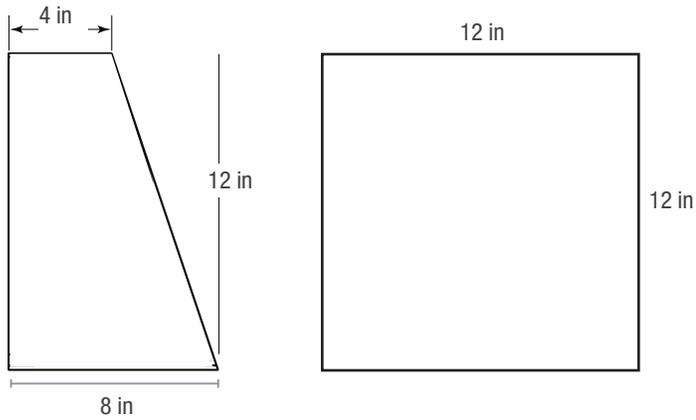
8" depth of fixture bottom lens side tapers to 4" top
