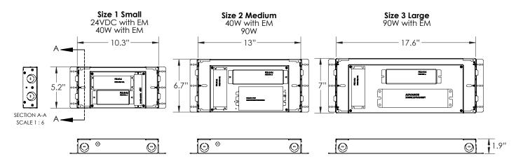
BBUX - BATTERY BACK-UP & LED DRIVER REMOTE (OUTDOOR), IP67, IK10, NEMA 4X, -20°C to +55°C, 30' MAX Distance with 12AWG (w/UNV Option Only)
