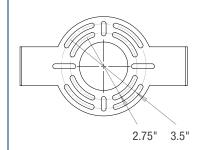
j-box mounting plate: mounts flush to surface and is included with fixture
