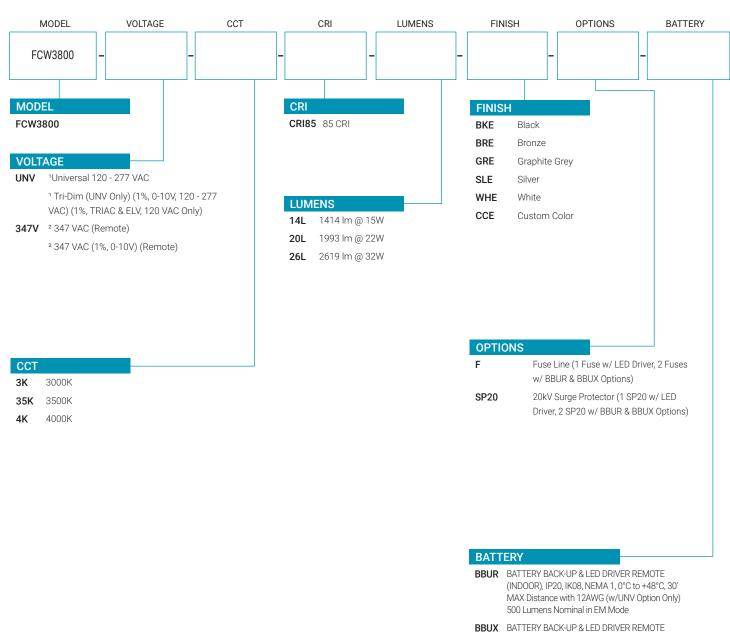
(OUTDOOR), IP67, IK10, NEMA 4X, -20°C to +55°C, 30' MAX Distance with 12AWG (w/UNV Option Only) 600 Lumens Nominal in EM Mode
