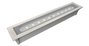
FCD7001 Linear Inground Uplight is ETL listed for wet locations. Housing is marine grade, corrosion resistant, heavy walled, high pressure aluminum construction with 316 machined brushed stainless steel trim (aluminum well housing included). Lens is impact resistant, clear, tempered glass. Reflector is precision formed semi-specular aluminum for maximum reflectance with LED.
