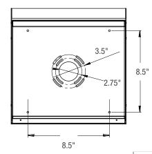
mounts flush to j-box surface and is included with luminaire
